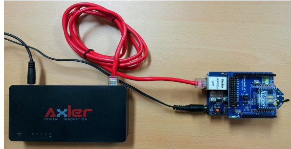
Figure 2. Base station connected to Ethernet router consisting of an Arduino UNO, an Ethernet Shield and XBee ZB module
